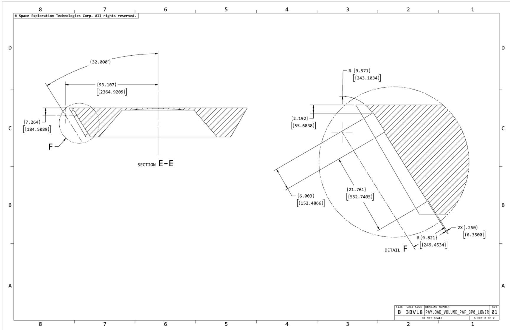
Figure 12-7: Payload lower volume, with 1,575-mm PAF (2 of 2)
