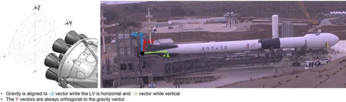
Figure 2-4: Falcon vehicle coordinate frame
