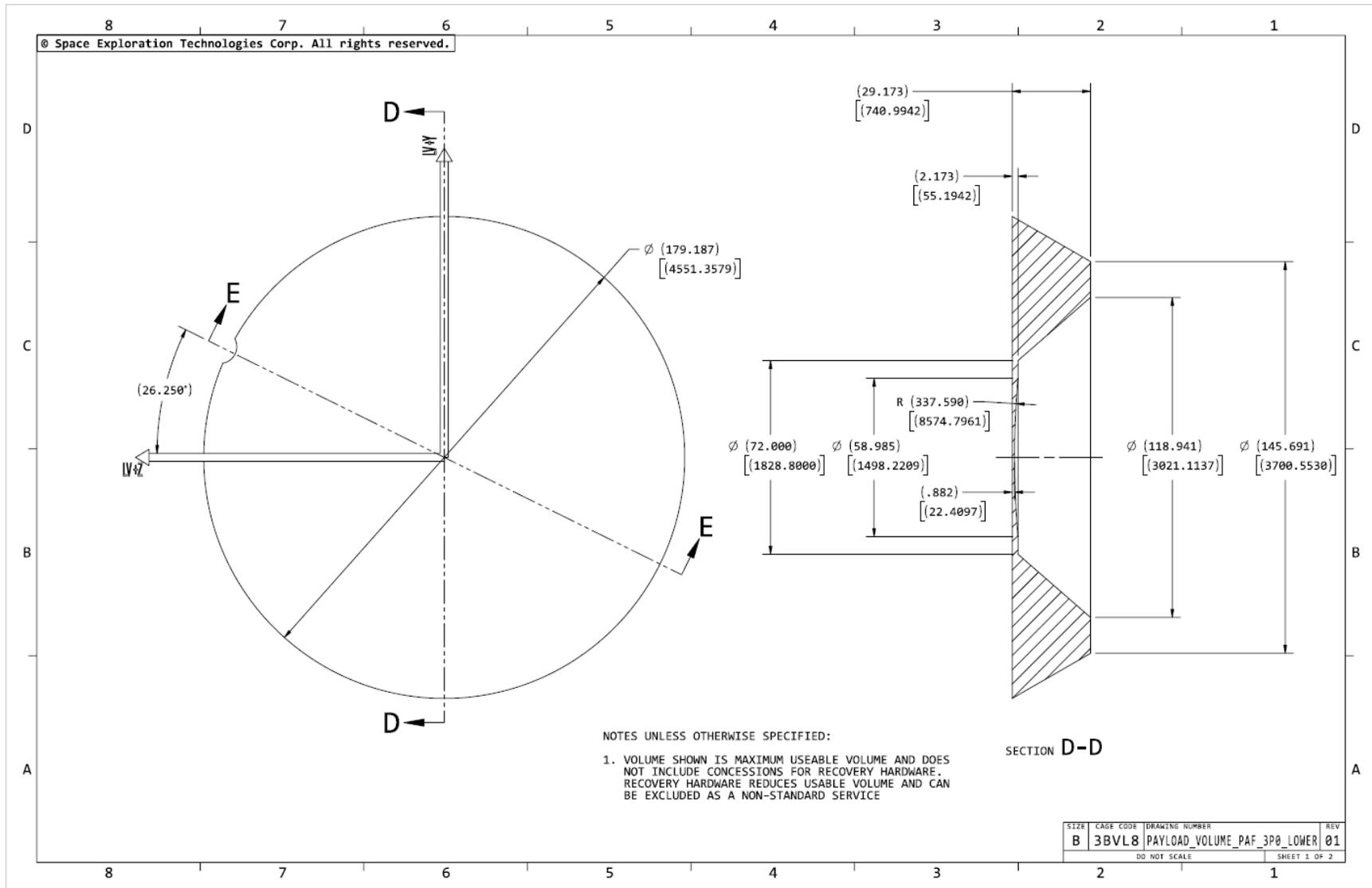
Figure 12-6: Payload lower volume, with 1,575-mm PAF (1 of 2)
