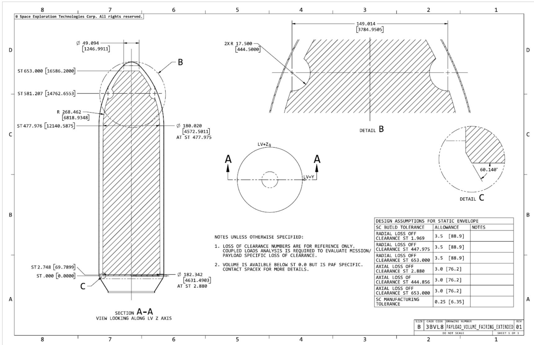
Figure 12-10: Falcon extended fairing with payload static envelope
