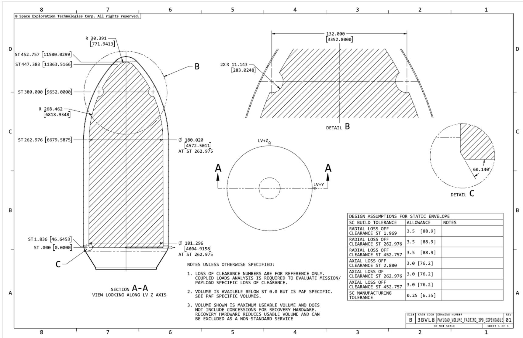
Figure 12-5: Payload static envelope (standard Falcon fairing)
