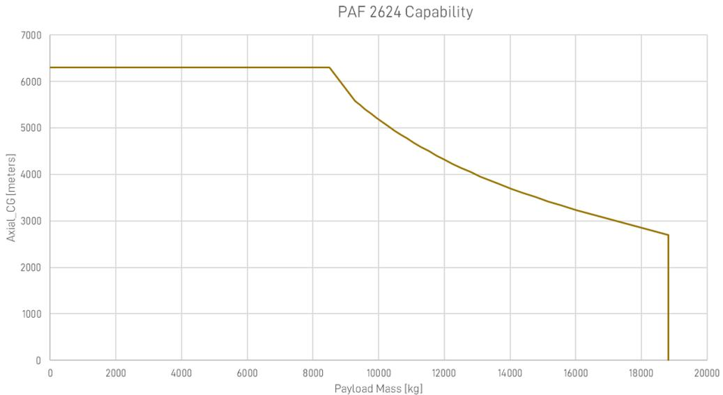
Figure 3-4: Allowable center-of-gravity height above the 2,624-mm plane
