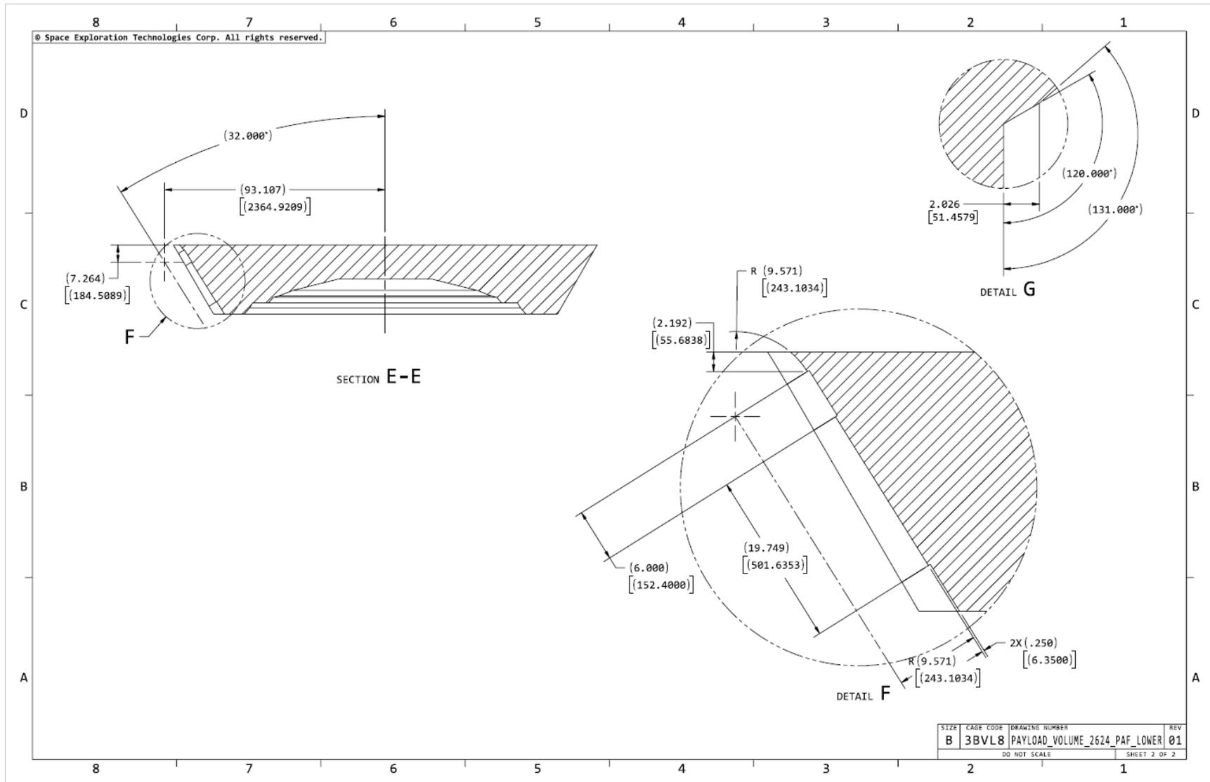
Figure 12-9: Payload lower volume, with 2,624-mm PAF (2 of 2)
