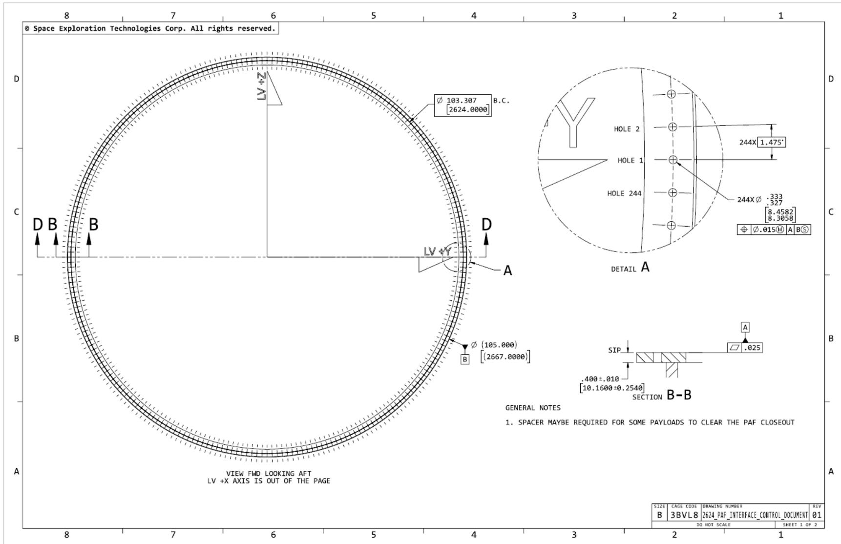
Figure 12-3: 2,624-mm interface drawing (interface plane details)
