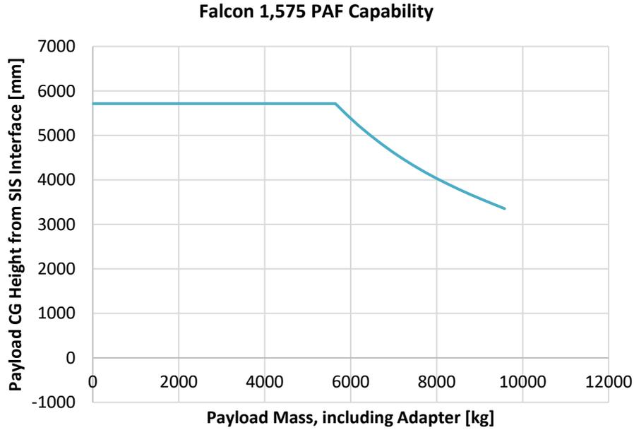
Figure 3-3: Allowable center-of-gravity height above the 1,575-mm plane
