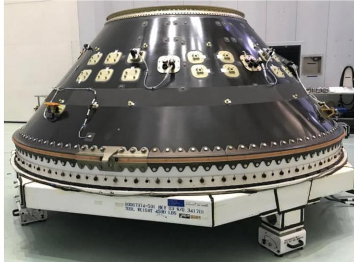
**Figure 3-1: SpaceX 1,575-mm payload attach fitting**
