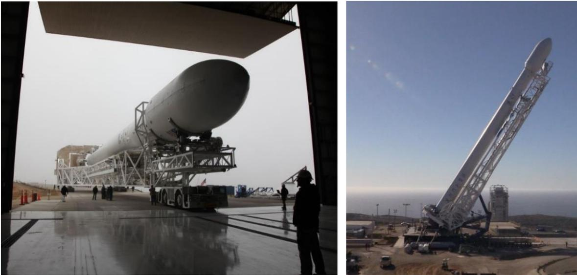
Figure 8-9: Launch vehicle rollout and erection
