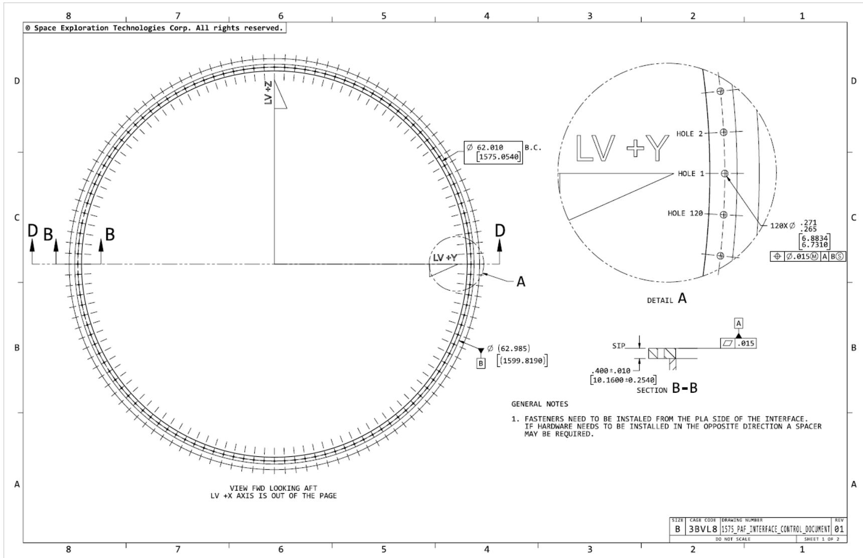
Figure 12-1: 1,575-mm interface drawing (interface plane details)
