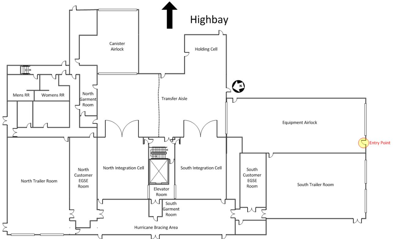
**Figure 8-4: CCSFS PPF West Bay floor plan**
